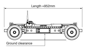
AGITO Sports - Multi terrain/dolly wheels Wheel diameter =185mm Ground clearance =78mm
